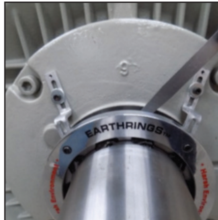
15) Use 1mm Feeler gauge to check Earthring has a minimum of 1mm gap from the shafts shoulder, plus also check that Earthring is vertically straight at 90 degree angle / parallel with the shaft and grease cover / endshield.
