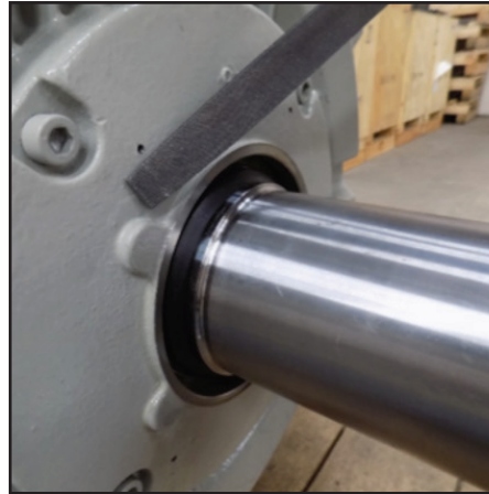
12) If you happen to break the tap, do not panic, file down the broken tap until it is flush with the grease cover, then drill a new hole 3 or 4mm below or above the old hole (Bracket has slide-groove that will allow for this adjustment).
