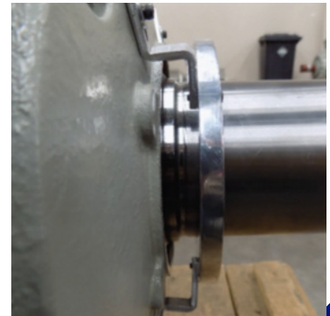
15) Use 1mm Feeler gauge to check Earthring has a minimum of 1mm gap from the shafts shoulder, plus also check that Earthring is vertically straight at 90 degree angle / parallel with the shaft and grease cover / endshield.
