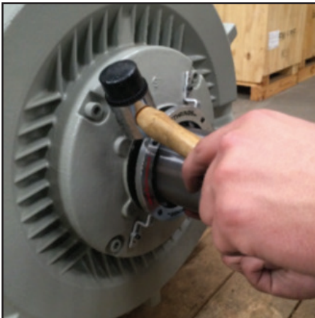
14) Move or tap Earthring so it is evenly positioned around shaft (1mm clearance over shaft), use feeler gauge 0.9mm or 0.8mm thickness to ensure even gap all around shaft.
